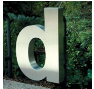
Water-jet cut & welded channel SII St letters
