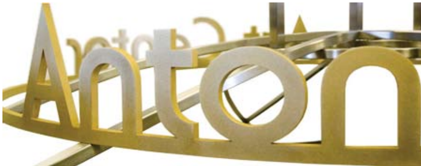
1/2" Waterjet cut bronze graphics mechanically mounted to a tig welded ring.
