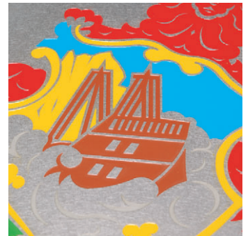
Waterjet cut, etched multi-coloured infilled st.stl. plate
